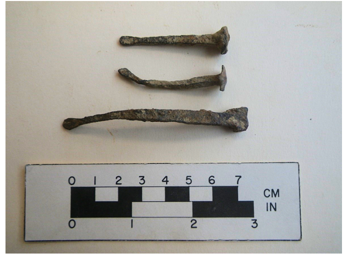
Examples of hand-wrought nails recovered from an archaeological site in Fairfax County.
